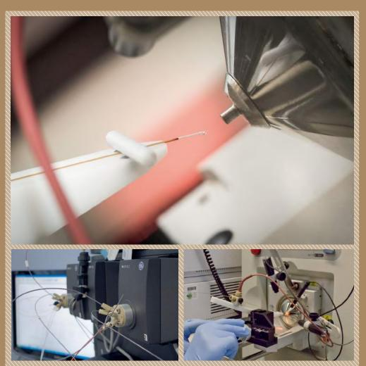
Top: Nano capillary chromatography column (tip diameter ≈0.008 mm) interfaced with electrospray ionization source of mass spectrometer. Left: High Performance Liquid Chromatography (HPLC) system for separation of peptides and proteins. Right: Setting up peptide analysis on a LTQ-Orbitrap mass spectrometer.
