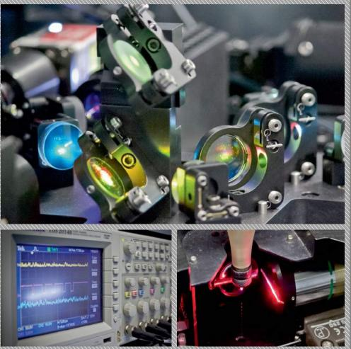
Top: A complex mirror system leads the laser beams to the interrogation point where the laser intersects with the samples.
