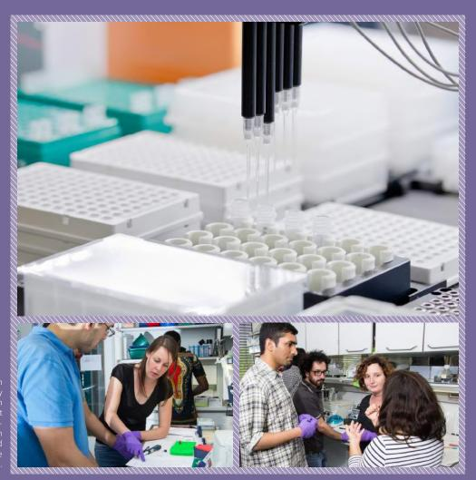
High throughput data production with the latest sequencing technology supporting a broad range of research applications. **Top**: high throughput sample preparation for transcriptome analysis of 96 samples using an automated platform and customized protocols. **Bottom**: course for sample preparation for deep sequencing.
