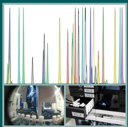
lop: Metabolites were measured by GC-MS. Then peaks were automatically detected and integrated by our in-house data processing. Left: <sup>32</sup>C tracing samples in autosampler awaiting measurement on GC-MS. Right: Sample prep for quantification of polar metabolites on LC-MS.
